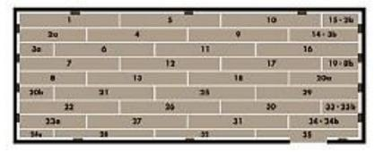
Snap a chalk line at the starting point to maintain alignment. Use planks mixed in from four or five cartons to achieve the ideal random pattern.
